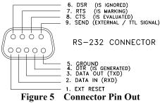
The balance will not output any information under any circumstances unless pin 8 (CTS) is held in an ON state (+3 to +15 VDC). Interfaces not utilizing the CTS handshake may tie pin 8 to pin 7 or pin 8 to pin 4 to defeat it.
