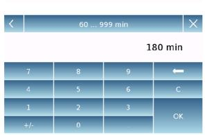
To change the auto-calibration range, tap the "Calibration Range" key and set the desired range between 60 and 999 minutes.
