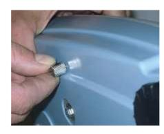
**Level** the balance by adjusting the legs on the front of the balance.
