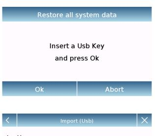
Insert the USB stick into the USB port on the left side of the device, and press the "OK" key.
