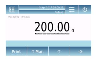
If you work with weighing boxes, first zero the balance. Place the container and press the "-T-"key.
