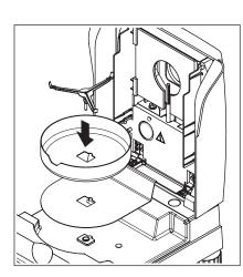
First lay the heat shield in the sample chamber. Then place the draft shield (can only be mounted in one position) and after that the sample pan support in position. Turn the sample pan support until it engages. In the engaged position the rear arm of the sample pan support lies exactly along the length of the instrument.
