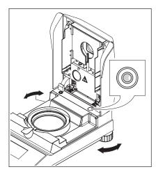
For exact horizontal positioning, the Moisture Analyzer has a level indicator (level) and 2 leveling screws. When the air bubble in the level indicator is exactly in the center, the instrument is standing perfectly horizontally. To level it, proceed as follows:
