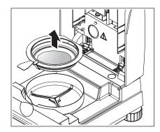
Carefully remove the sample pan handler from the sample chamber.
