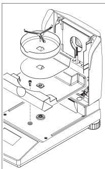
The draft shield, sample pan support and heat shield can be removed for cleaning without tools.
