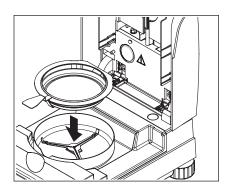
Place the empty sample pan in the sample pan handler (this is possible without tilting the sample pan if you insert this in the pan handler **from the side** directly below the round flange). Place the sample pan handler in the draft shield. Ensure that the tongue of the pan handler fits exactly in the slot of the draft shield. The sample pan must lie flat in the pan holder.
