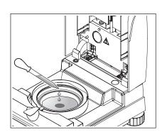
Wet the specimen sample with a few drops of water, so that the displayed weight is at least 0.5 grams (required minimum weight of sample). Note:The drying process cannot start until the minimum sample weight has been reached.
