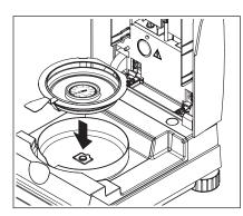
Insert the temperature adjustment set in the sample pan handler.
