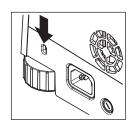
For protection against theft, your Halogen Moisture Analyzer is fitted with a socket for an antitheft device. Together with a lockable steel cable like those used to protect portable computers against theft, the socket can be used to secure the instrument. You can obtain a suitable antitheft cable from your METTLER TOLEDO dealer.
