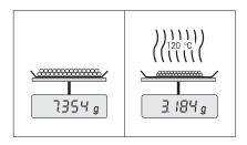
In principle, your instrument thus comprises two instruments: a precision balance and a heating module. In contrast to other thermogravimetric methods (drying oven, infrared, microwave), the Halogen Moisture Analyzer operates with a halogen heating module. This ensures fast heating of the sample and thus guarantees rapid availability of the measurement results.
