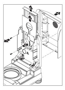
To dismantle the heating module the four screws (1) must be unscrewed. A screwdriver is needed for this purpose (Torx T-20).
