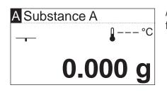
After it has been switched on, the instrument performs a self-test. Wait until the display shown opposite appears.
