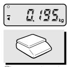
4Remove container and commodity, then the display will show the weight of the container with "-" symbol.
